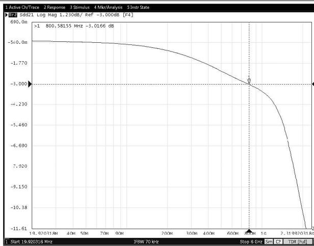
Figure 31. Data Transmission Characteristics vs Frequency (TPS25830-Q1)
