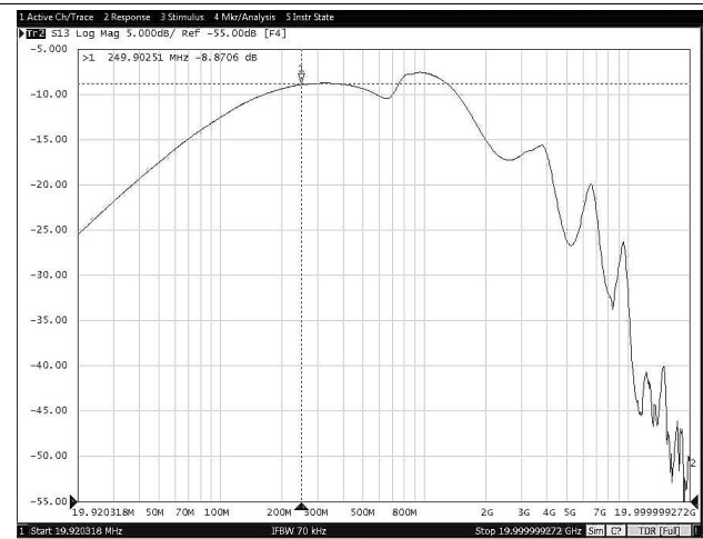
Figure 32. Off-State Data-Switch Isolation vs Frequency (TPS25830-Q1)
