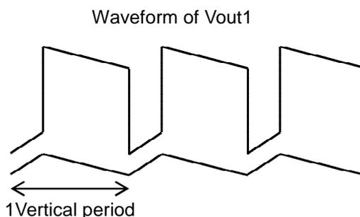
SAG correction circuit generates a low frequency component signal amplified to Vout terminal. Changes of the luminance signal will be low-frequency components, if you want to output a large signal luminance changes. Therefore, generate correction signal of change of a luminance signal to Vout pin. At this time, signal is over the dynamic range of Vout pin. This may cause a lack of sync signal, and waveform distortion.
