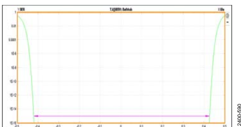
Figure 128. Bathtub, External 100 \Omega Terminations at 10 Gbps
