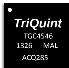
28-pin 5x5mm QFN package
