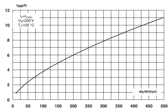
**Figure 5. Reverse recovery time versus  $dI_F/dt$  (typical values)**
