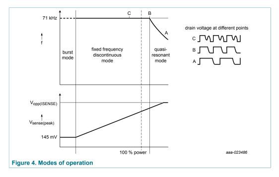
Fixed-frequency DCM mode is the primary mode of operation. It is based on an accurate oscillator, which sets the nominal switching period. When the oscillator time-period has completed and transformer demagnetization is detected at the AUX pin, a new switching cycle is started.
