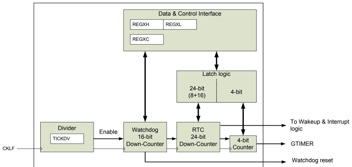
Figure 70. Watchdog and wakeup functions block diagram
