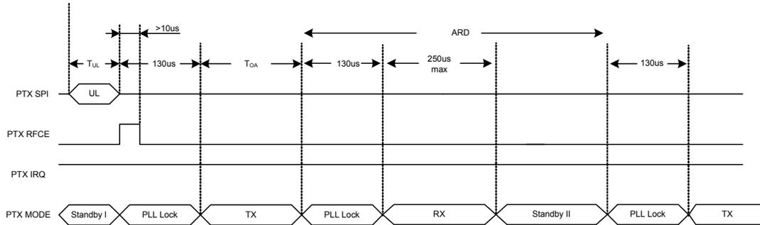
Figure 18. Timing of Enhanced ShockBurst™ when the first ACK packet is lost (2Mbps)
