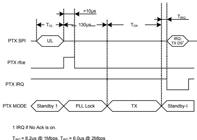
Figure 16. Transmitting one packet with `NO_ACK` on
