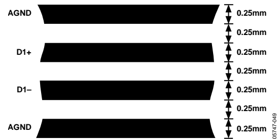
Figure 61. Arrangement of Signal Tracks
