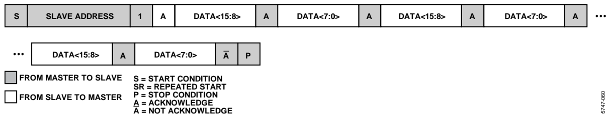
Figure 54. Reading Three Lots of Two Bytes of Data from the Conversion Result Register
