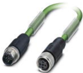
Bus system cable, Ethernet CAT5 (100 Mbps), 4-position, PVC/PVC, green RAL 6018, shielded, Plug straight M12, D-coded, on Socket straight M12, D-coded, cable length: 20 m
