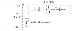
"DO NOT connect "DIM- to -V"
