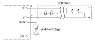
"DO NOT connect "DIM- to -V"
