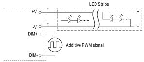
"DO NOT connect "DIM- to -V"
