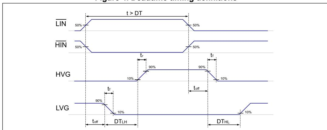
Figure 5. Deadtime and interlocking waveforms definition
