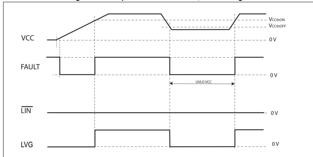
**Figure 7. VCC power ON and UVLO, HVG timing<sup>(a)</sup>**
