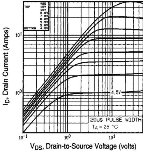
Fig. 1 - Typical Output Characteristics,  $T_A = 25\text{ °C}$
