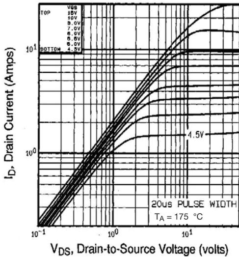
Fig. 2 - Typical Output Characteristics,  $T_A = 175\text{ °C}$
