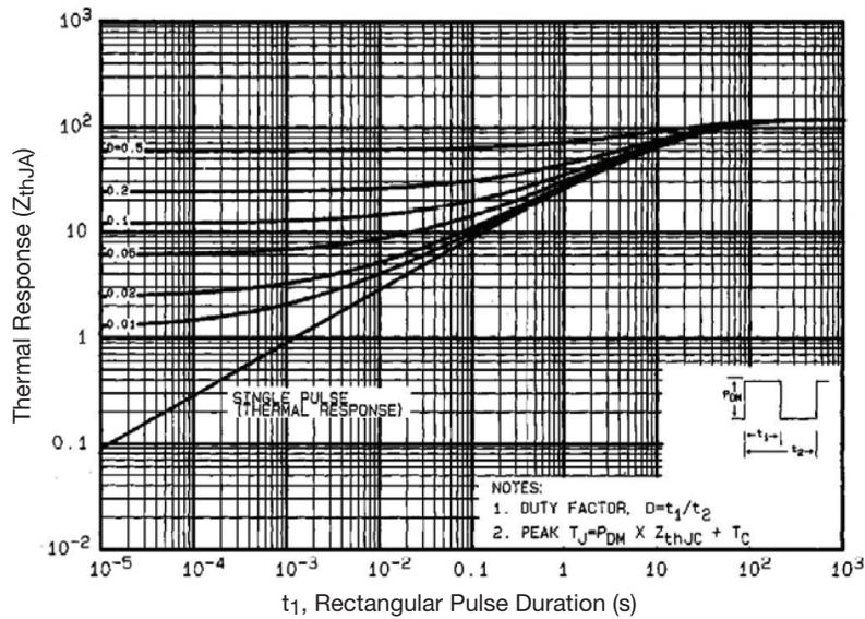
Fig. 11 - Maximum Effective Transient Thermal Impedance, Junction-to-Ambient
