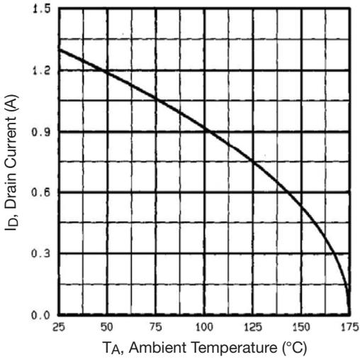
Fig. 9 - Maximum Drain Current vs. Ambient Temperature
