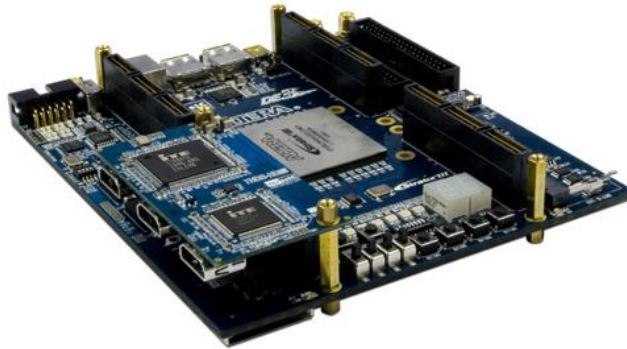
Figure 1-2 Connect HDMI daughter board to DE3 board
