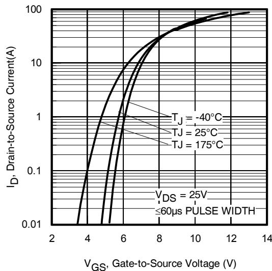
**Fig. 5.** Transfer Characteristics
