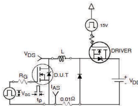
**Fig 18a.** Unclamped Inductive Test Circuit
