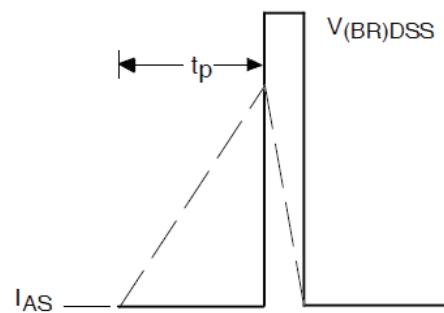
**Fig 18b.** Unclamped Inductive Waveforms
