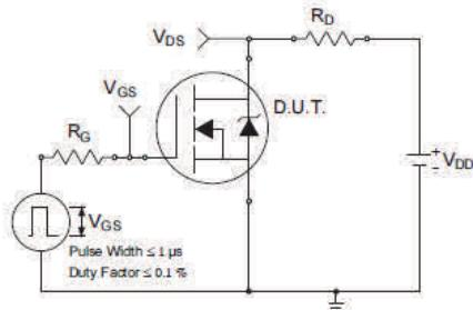
**Fig 20a.** Switching Time Test Circuit
