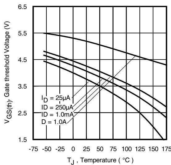
**Fig. 7** Typical Threshold Voltage vs. Junction Temperature
