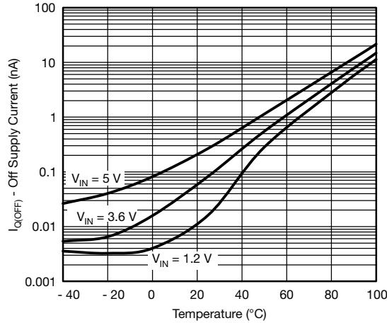
Figure 6 - Off Supply Current vs. Temperature
