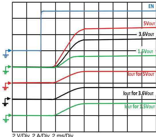
**Figure 20 - Typical Turn-on Delay, Rise Time**
