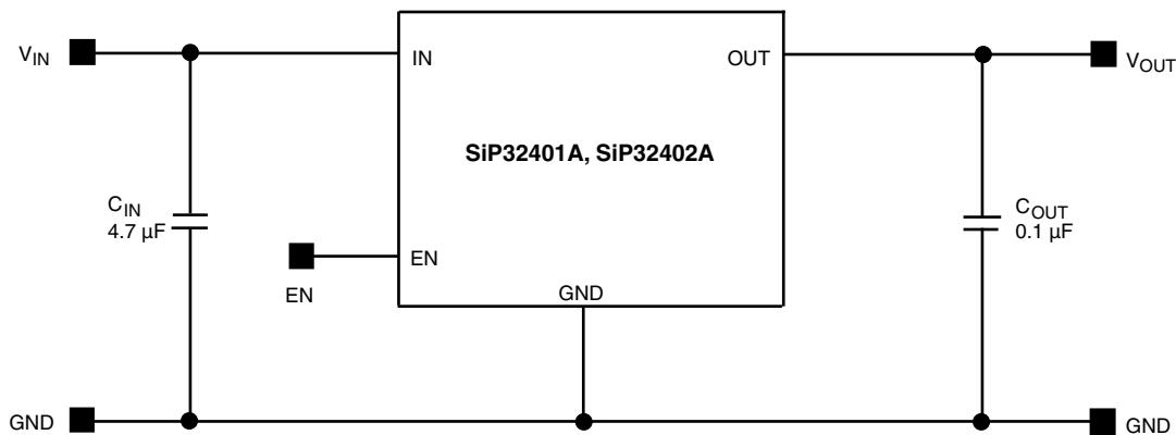
Figure 1 - SiP32401A, SiP32402A Typical Application Circuit
