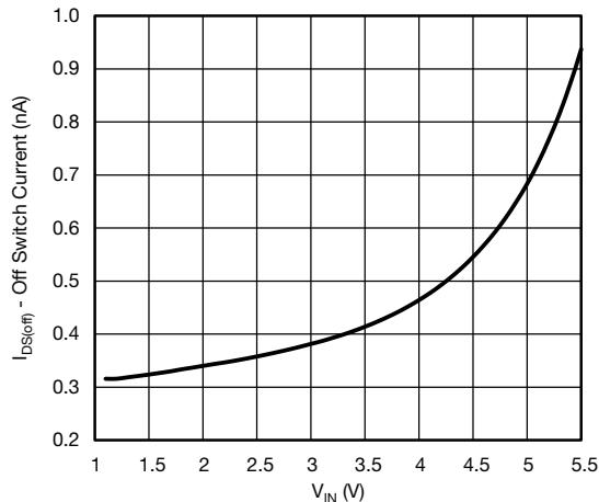
**Figure 7 - Off Switch Current vs. Input Voltage**
