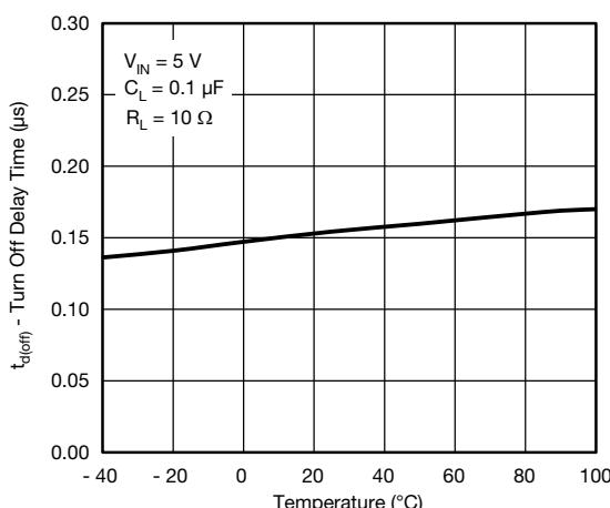
**Figure 17 - Turn-Off Delay Time vs. Temperature**
