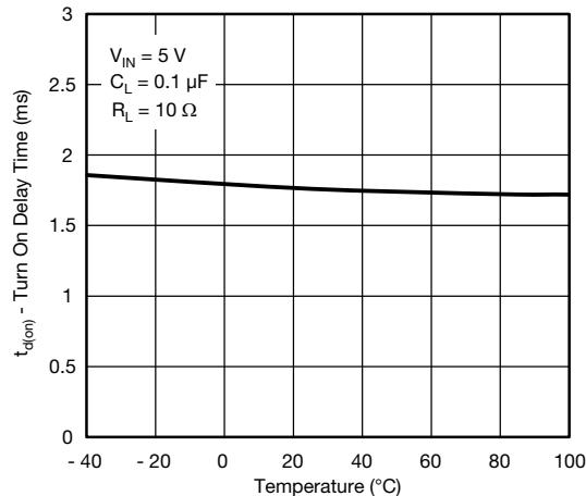
**Figure 16 - Turn-on Delay Time vs. Temperature**
