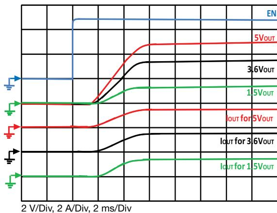
**Figure 18 - Typical Turn-on Delay, Rise Time**
