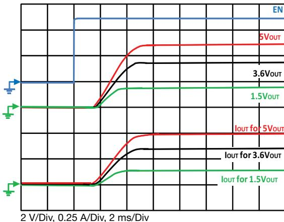
**Figure 19 - Typical Turn-on Delay, Rise Time**
