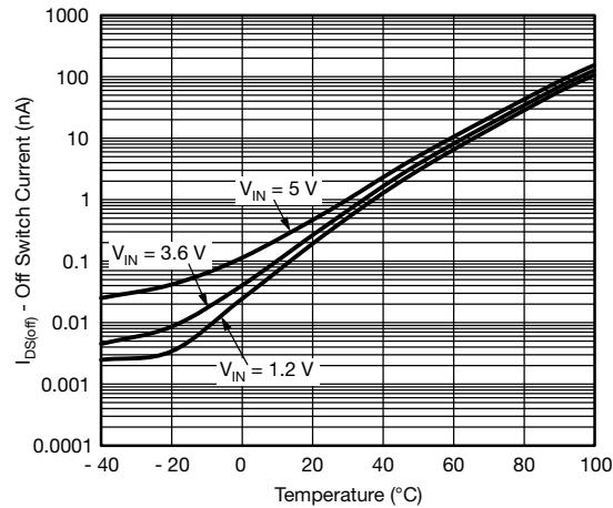
**Figure 10 - Off Switch Current vs. Temperature**
