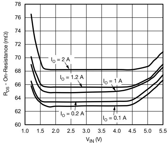
**Figure 8 - R<sub>DS(on)</sub> vs. V<sub>IN</sub>**
