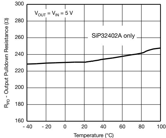
**Figure 12 - Output Pull Down vs. Temperature**
