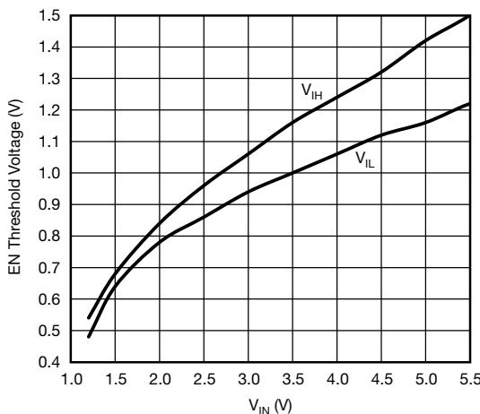
**Figure 15 - EN Threshold Voltage vs. Input Voltage**
