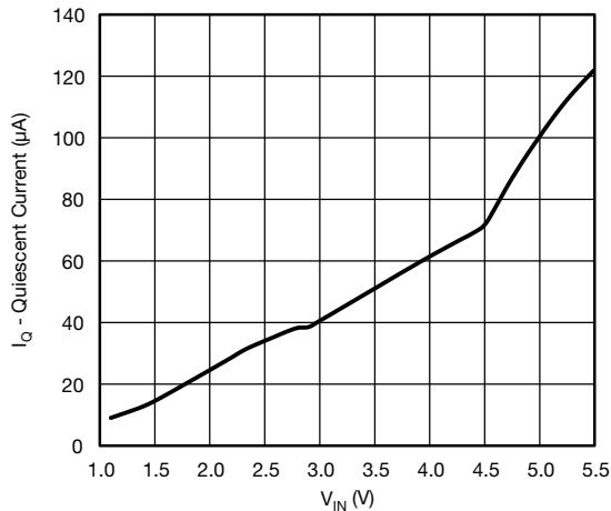
Figure 3 - Quiescent Current vs. Input Voltage
