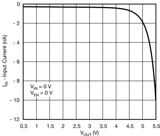
**Figure 13 - Reverse Blocking Current vs. Output Voltage**
