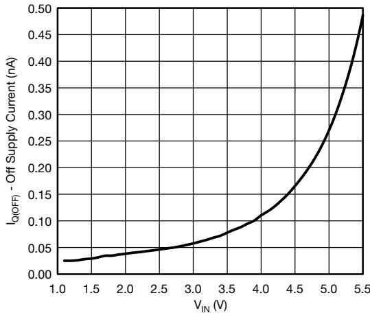
Figure 4 - Off Supply Current vs. Input Voltage
