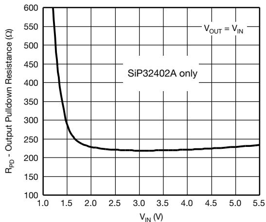
**Figure 9 - Output Pull Down vs. Input Voltage**
