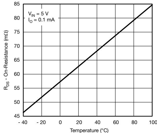
**Figure 11 - R<sub>DS(on)</sub> vs. Temperature**
