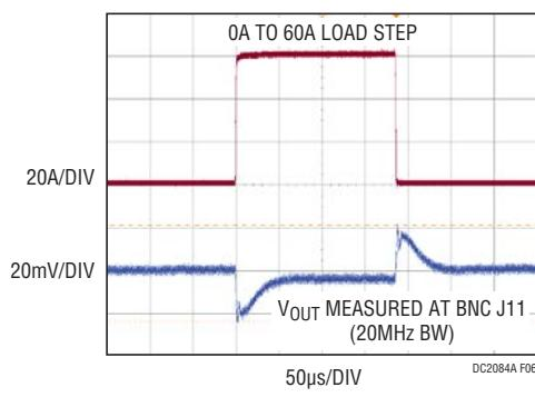
Figure 6. Transient Response at  $V_{IN} = 12V$ ,  $V_{OUT} = 1V$
