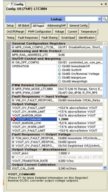
Then, click the "W" (PC to RAM) icon to write these register values to the LTC3884. After finishing this step, you will see the output voltage will change to 1.2V.
