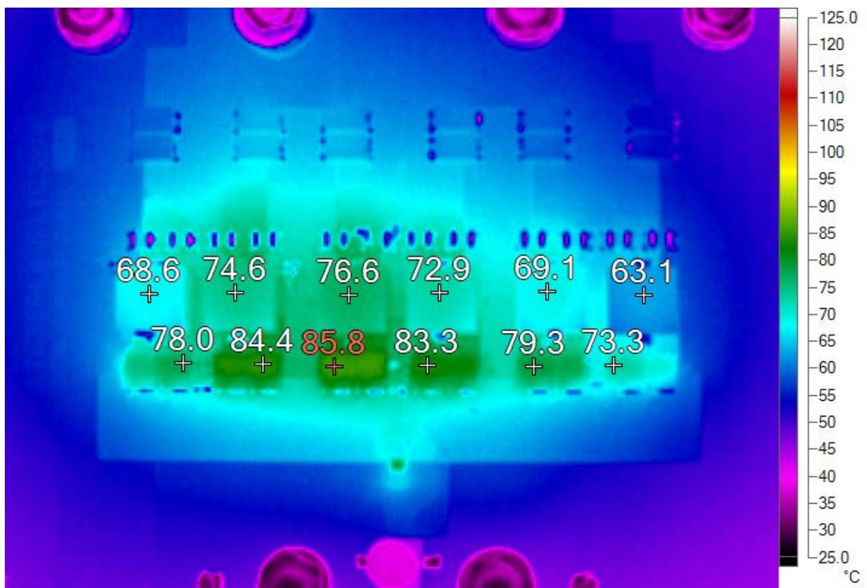
Figure 8. Thermal Performance at  $V_{IN} = 12V$ ,  $V_{OUT} = 1V$ ,  $I_{OUT} = 240A$ ,  $T_A = 23^{\circ}\text{C}$ , 200LFM Airflow
