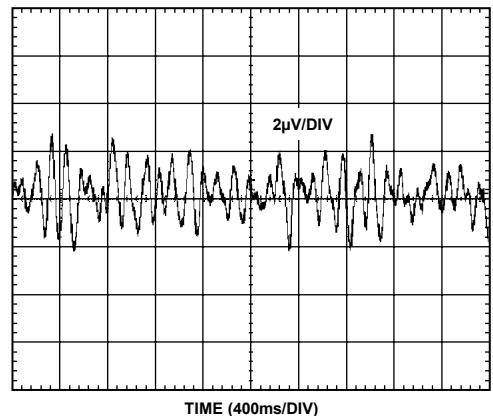
Figure 10. 1 Hz to 10 Hz Noise
