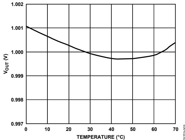
Figure 3. Typical  $V_{OUT}$  vs. Temperature
