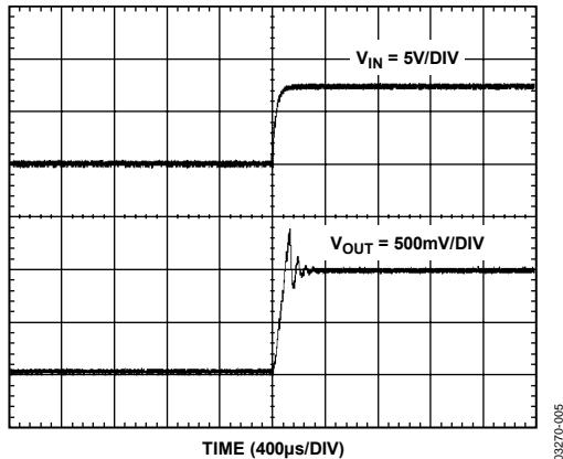
Figure 5. Turn-On Time with 1  $\mu$ F Input Capacitor
