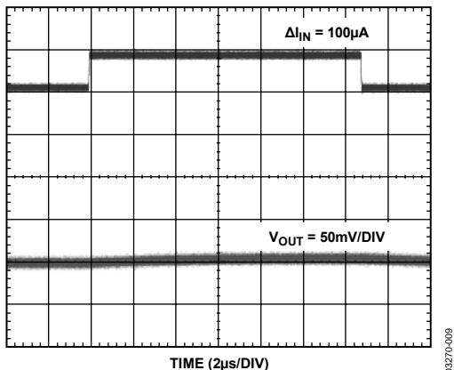
Figure 9. Output Response to 100  $\mu\text{A}$  Input Current Change
