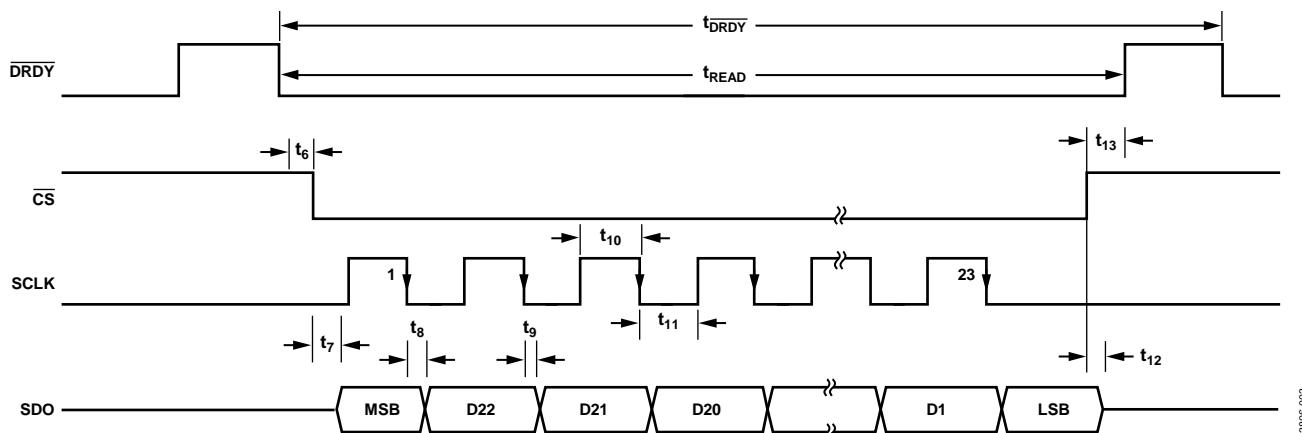
Figure 3. Serial Timing Diagram, Reading Data Using  $\overline{\text{CS}}$
