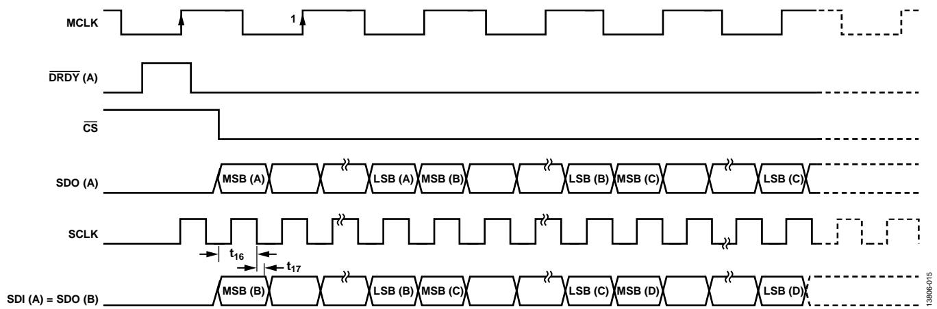
Figure 5. Daisy-Chain SDI Setup and Hold Timing
