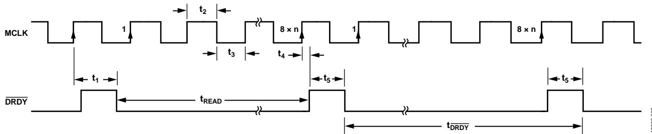
Figure 2.  $\overline{\text{DRDY}}$  vs. MCLK Timing Diagram,  $n = 4$  (Decimate by 32)
