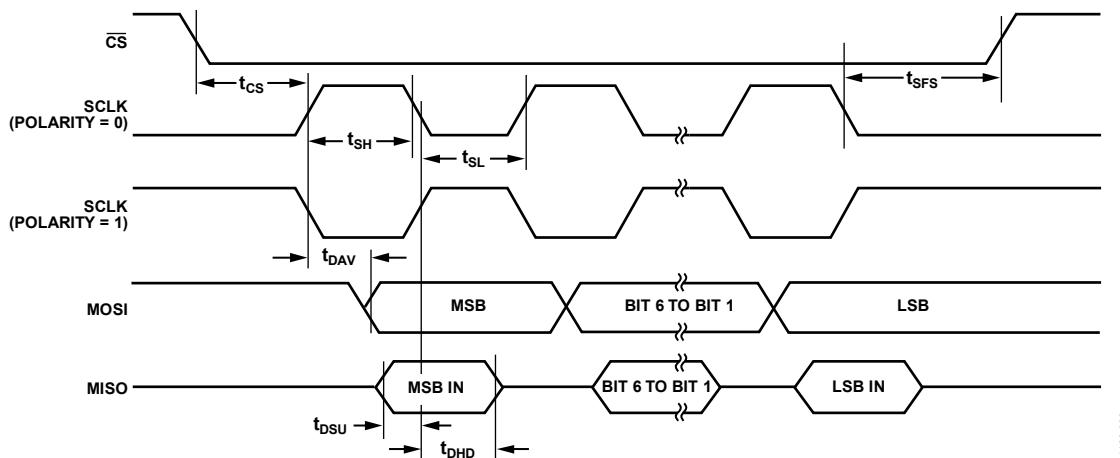
Figure 8. SPI Master Mode Timing (Phase Mode = 1)
