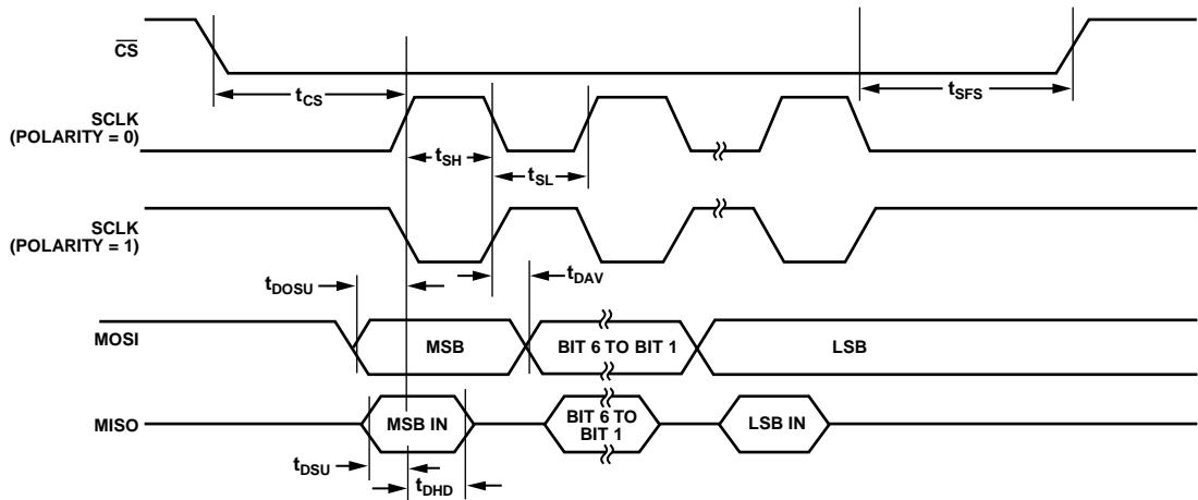
Figure 9. SPI Master Mode Timing (Phase = 0)
