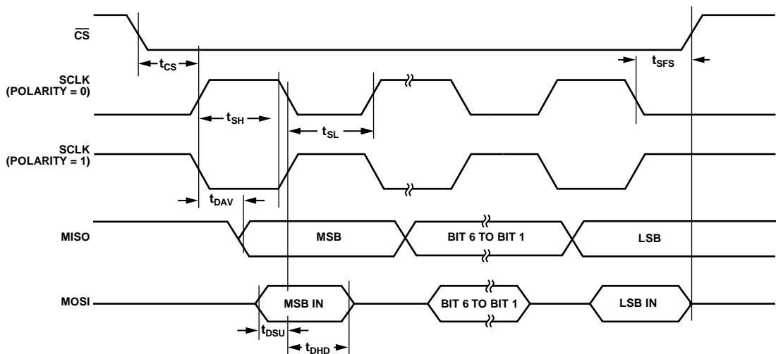
Figure 10. SPI Slave Mode Timing (Phase Mode = 1)
