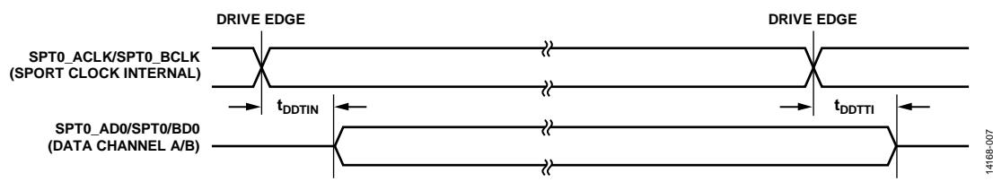
Figure 7. Enable and Three-State Serial Ports
