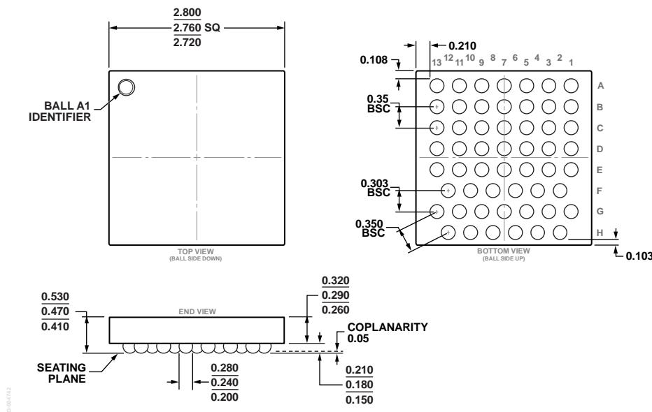
Figure 30. 54-Ball Wafer Level Chip Scale Package [WLCSP]
