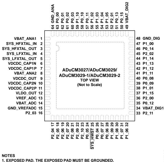
Figure 15. ADuCM3027/ADuCM3029/ADuCM3029-1/ADuCM3029-2 64-Lead LFCSP Configuration
