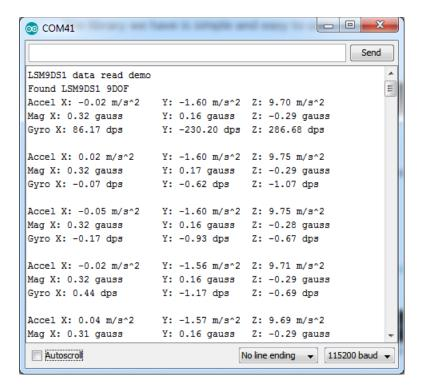
We suggest using this **Adafruit\_Sensor** interface as shown in this demo, since it will let you swap sensors without having to worry about units compatibility. Try twisting and moving the board around to see the sensors change value.
