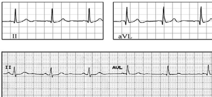
Fig. 3 Differential measurement of body (skin) surface potential to produce ECG trace
