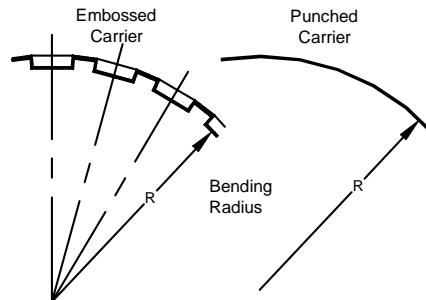
**Figure 5 – Reel Dimensions**
