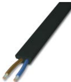
AS-Interface TPE flat-ribbon conductor with UL in black, for additional energy supply, 2 x 1.5 mm 2 , 25 m ring, with end clip for AS-Interface
