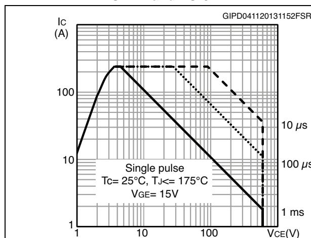
**Figure 13. Forward bias safe operating area for TO-3PF**
