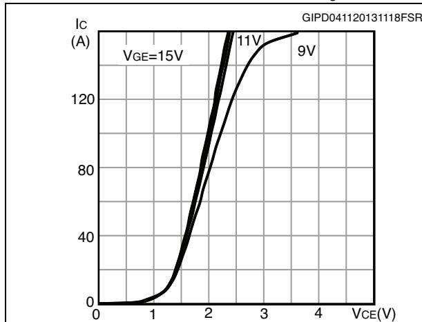
**Figure 7. Output characteristics ( $T_J = 175\text{ }^{\circ}\text{C}$ )**
