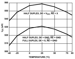
FIGURE 11. SUPPLY CURRENT vs TEMPERATURE
