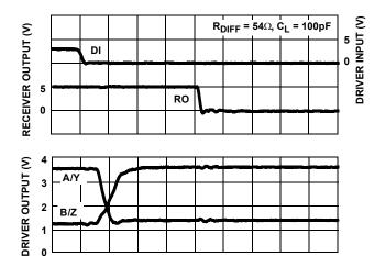
FIGURE 23. DRIVER AND RECEIVER WAVEFORMS, HIGH TO LOW (ISL83086E, ISL83088E)
