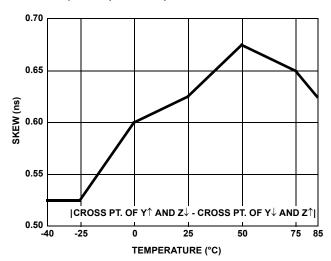
FIGURE 17. DRIVER DIFFERENTIAL SKEW vs TEMPERATURE (ISL83086E, ISL83088E)
