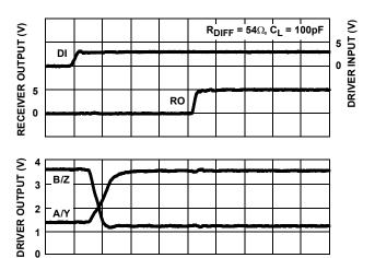
FIGURE 22. DRIVER AND RECEIVER WAVEFORMS, LOW TO HIGH (ISL83086E, ISL83088E)
