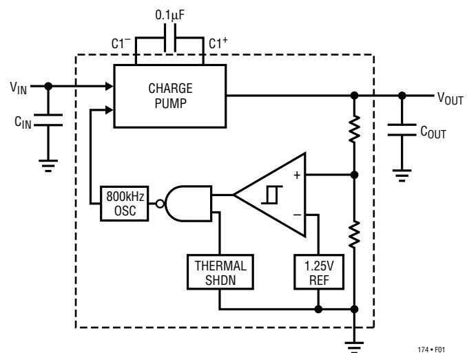
Figure 1. LTC1517-X Block Diagram
