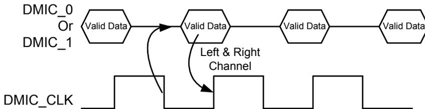
Figure 6. Stereo Digital Microphone Configuration
