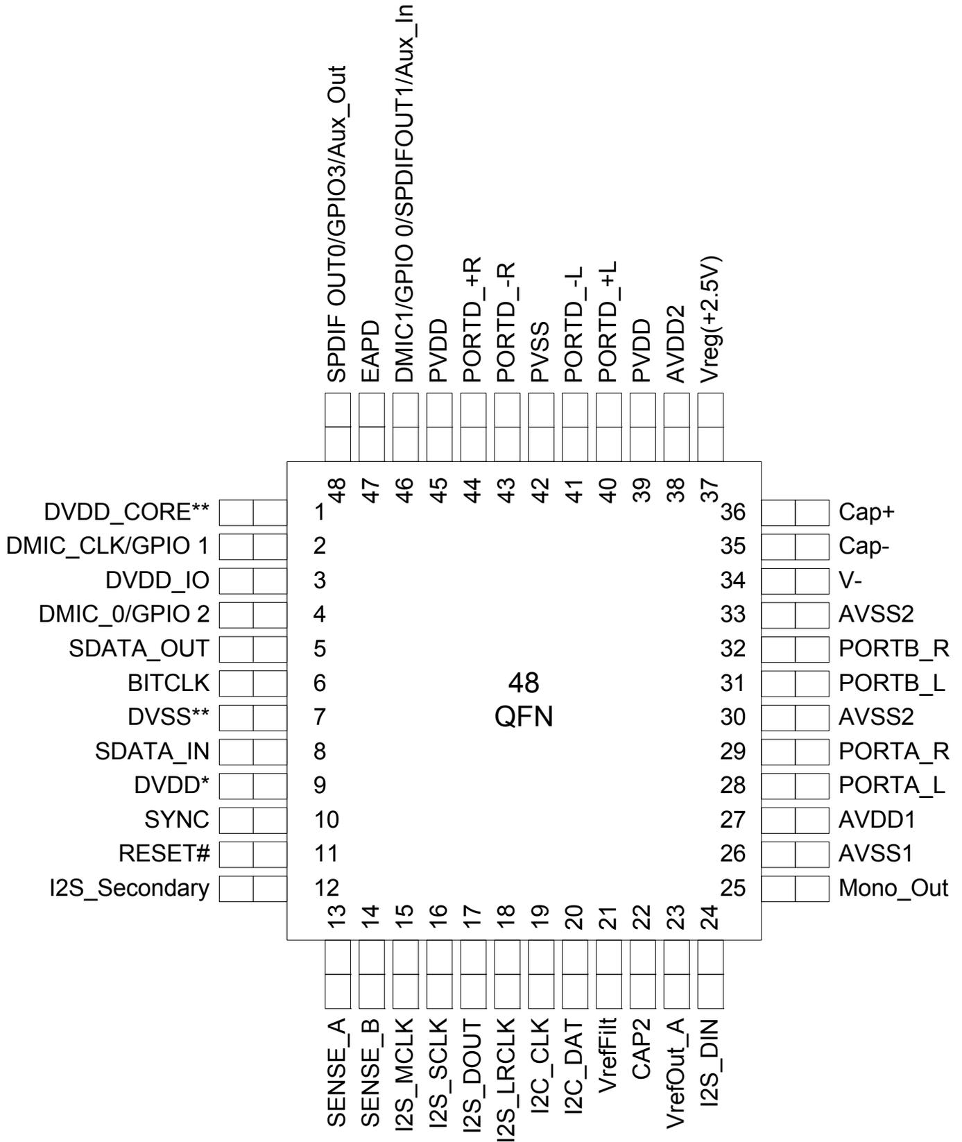
Figure 26. 48QFN Pin Assignment
