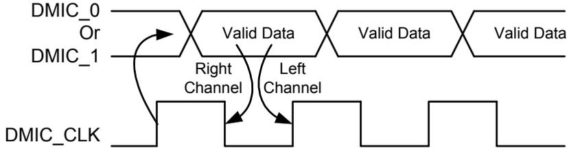
**Single "Left" Microphone, DMIC input set to mono input mode.**
