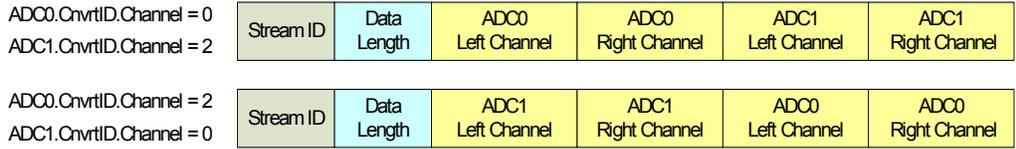
The following figure describes the bus waveform for a 24-bit, 48KHz capture stream with ID set to 1.
