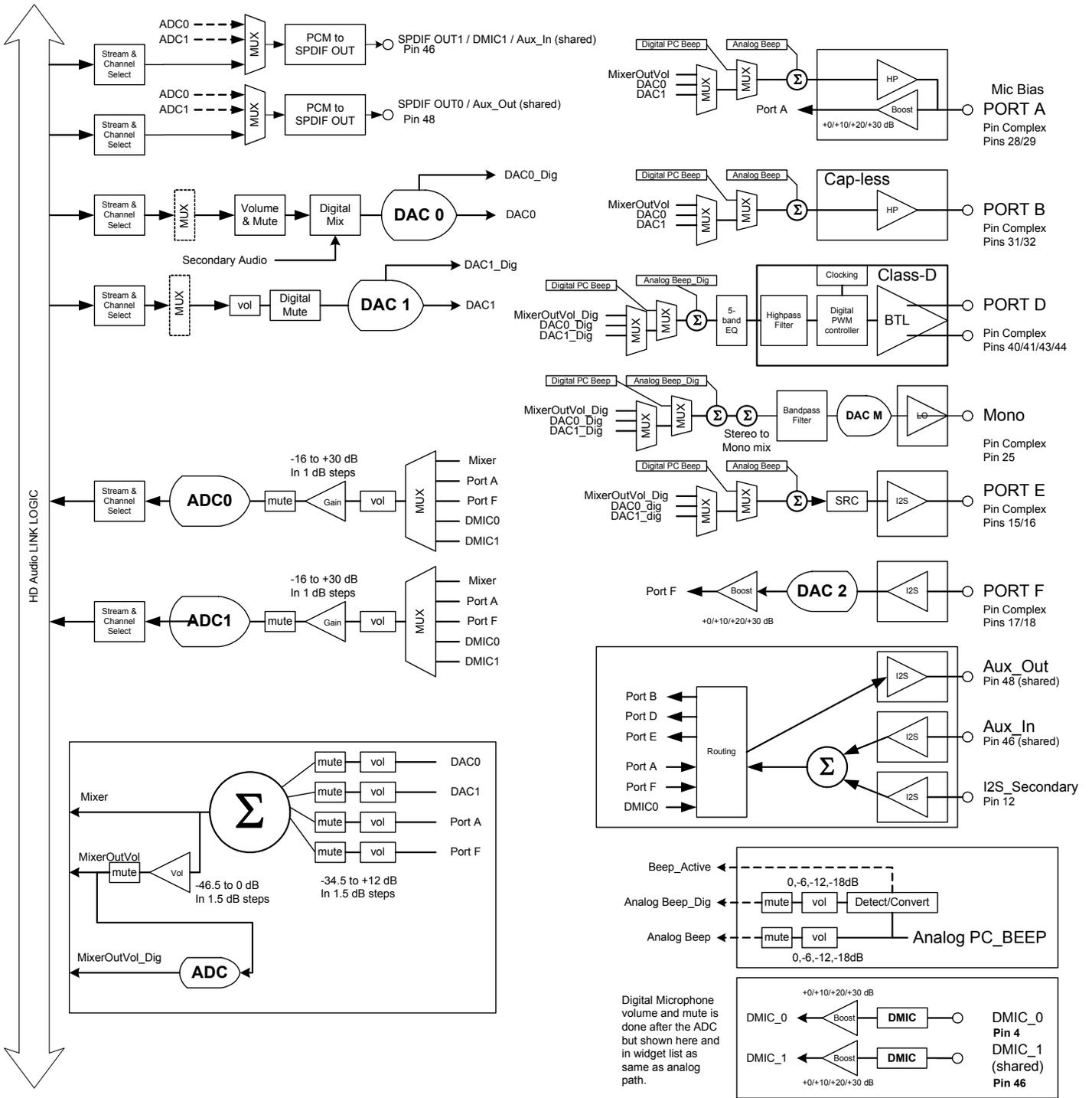
Figure 22. Functional Block Diagram
