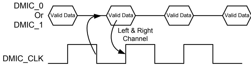
Figure 6. Stereo Digital Microphone Configuration
