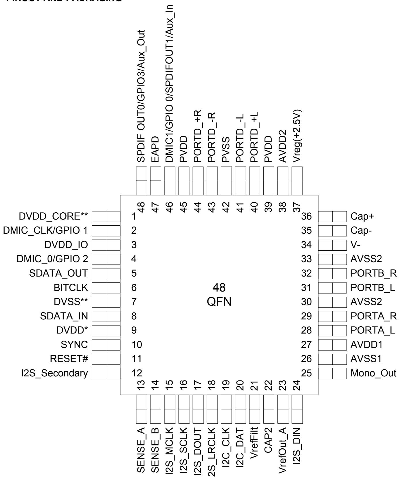
Figure 26. 48QFN Pin Assignment
