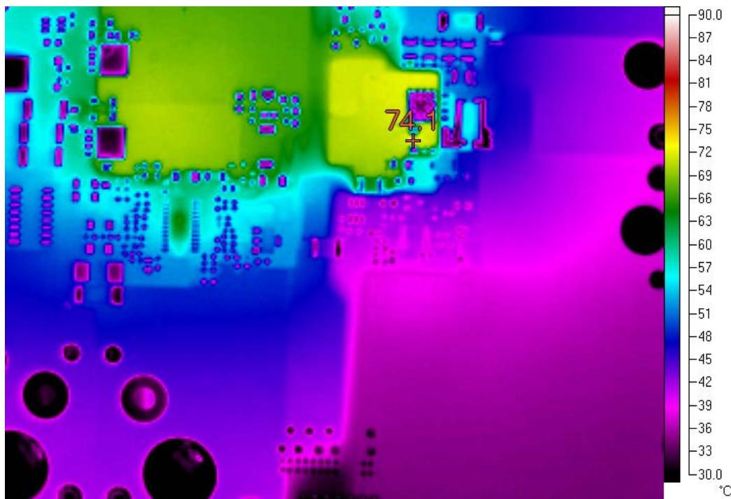
Figure 6. Thermal Map, Back Side at  $48V_{IN}$  and  $30A_{OUT}$  ( $T_A = 25^\circ C$ , 200LFM)
