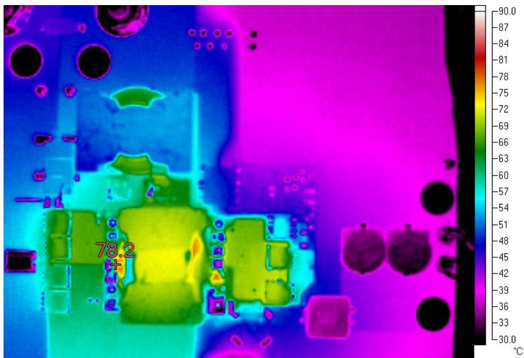
Figure 5. Thermal Map, Front Side at  $48V_{IN}$  and  $30A_{OUT}$  ( $T_A = 25^\circ C$ , 200LFM)
