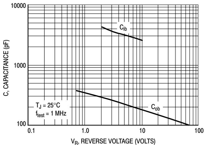
Figure 15. MJ21196 Typical Capacitance
