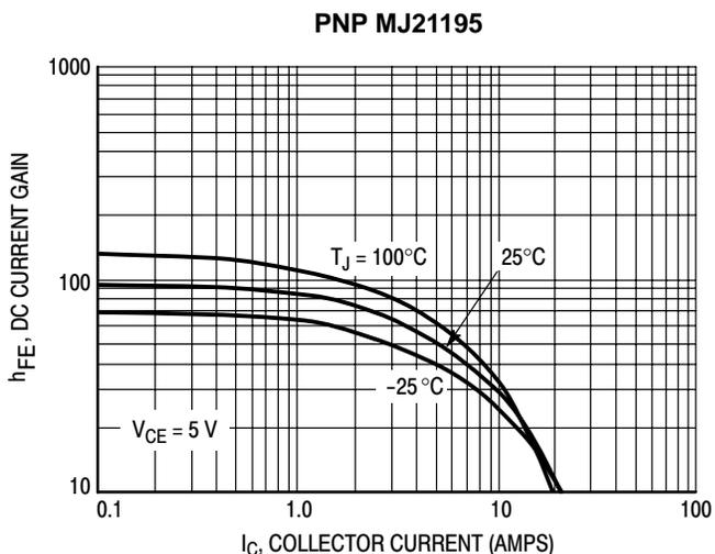
Figure 5. DC Current Gain,  $V_{CE} = 5\text{ V}$
