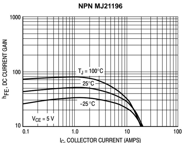
Figure 6. DC Current Gain,  $V_{CE} = 5\text{ V}$
