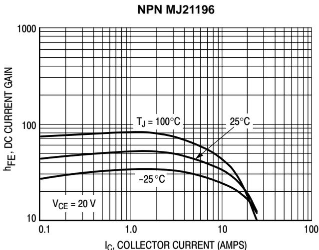
Figure 4. DC Current Gain,  $V_{CE} = 20\text{ V}$
