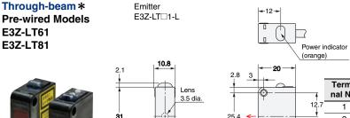
4 dia. vinyl-insulated round cable with 2 conductors (Conductor cross section: 0.2 mm² (AWG24), Insulator diameter:1.1 mm), Standard length: 2 m
