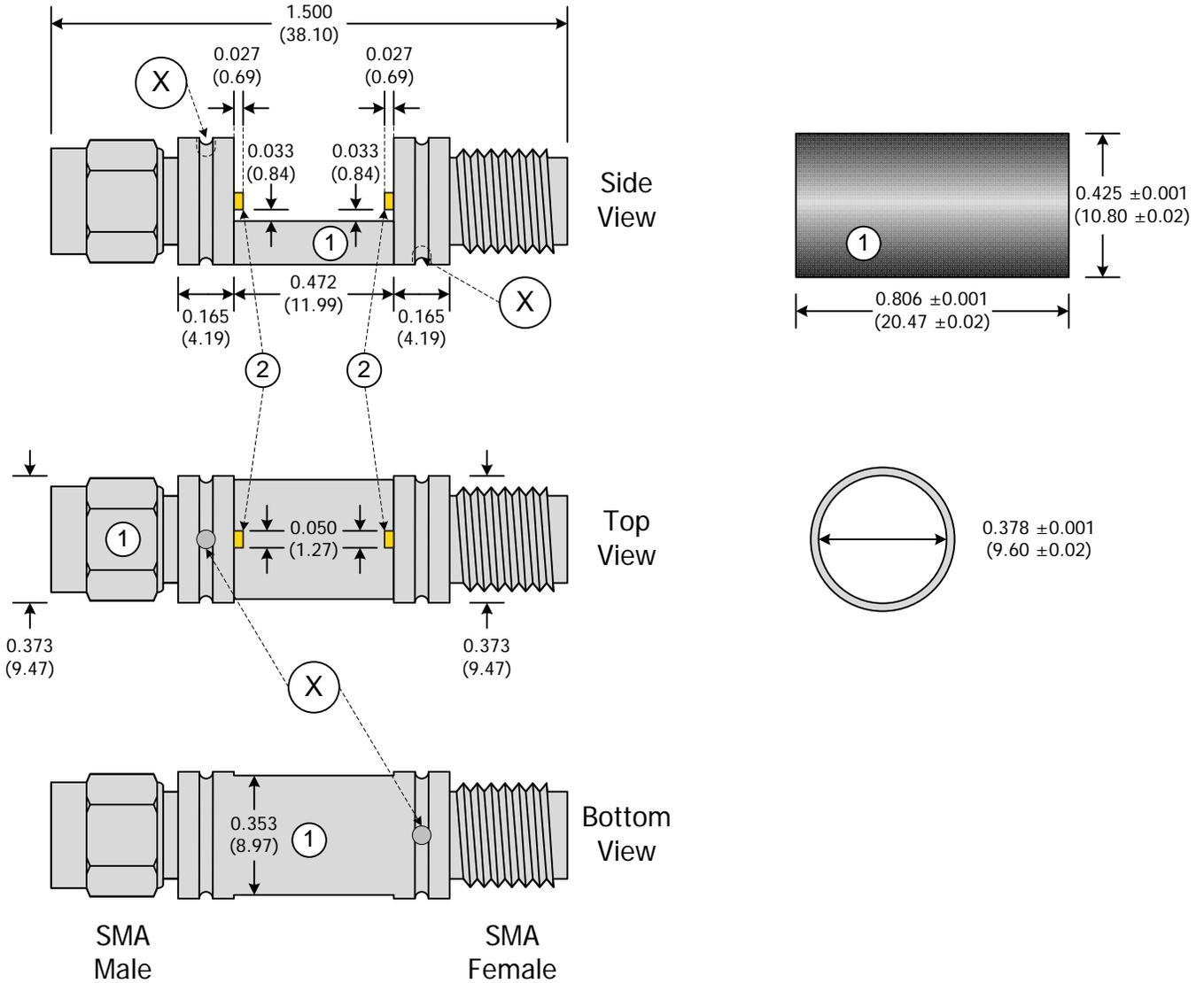
(X) Tooling Dimple, 2 Locations, Diameter 0.055 in (1.40 mm), Depth 0.055 in (1.40 mm)
