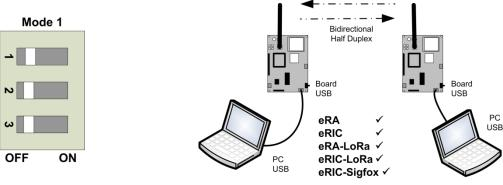
Set the Mode Switch to Mode1 (as shown).
