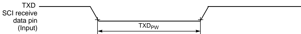
Figure 3-26 TXD Pulse Width
