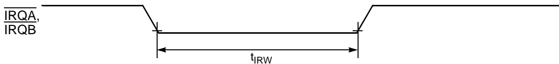
Figure 3-13 External Interrupt Timing (Negative-Edge-Sensitive)
