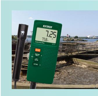
**Compact handheld Conductivity Meter with long life carbon rod combination electrode measures Conductivity, TDS and Temperature. Units of measure include  $\mu\text{S}/\text{cm}$ ,  $\text{mS}/\text{cm}$ ,  $\text{ppm}$ ,  $^{\circ}\text{F}$ , and  $^{\circ}\text{C}$ . The meter features three ranges for Conductivity and TDS plus adjustable Temperature compensation factor to maintain accuracy.**
