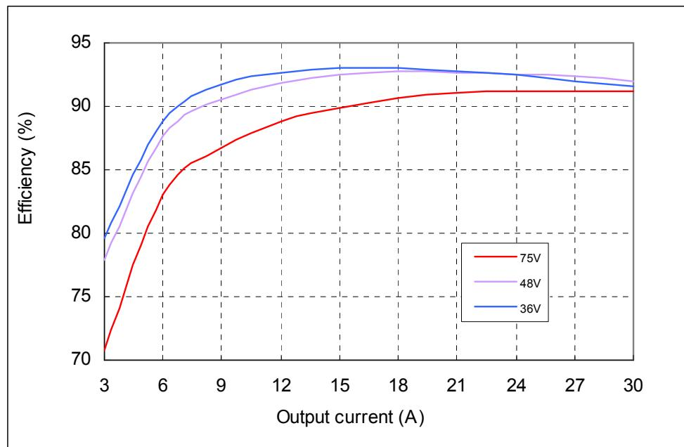
Figure 1 Efficiency vs. output current, T<sub>a</sub>=25°C, V<sub>o</sub>=3.3V
