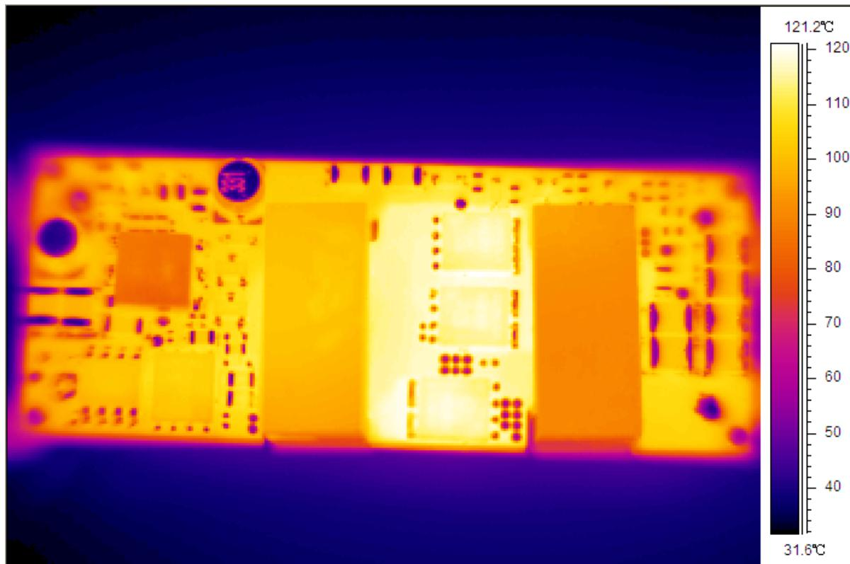
Figure 20 Thermal image, 48V<sub>in</sub>, 3.3V<sub>o</sub>, full load, room temperature, 100LFM (air flowing from pin 3 to pin 1)
