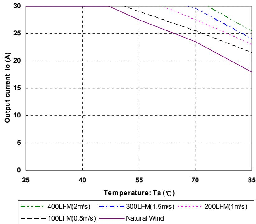
Figure 19 Output power derating, 48V<sub>in</sub>, air flowing across the converter from pin 3 to pin 1
