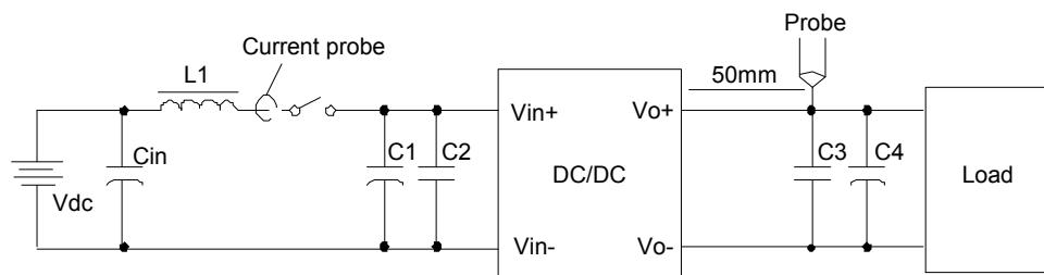
Figure 16 Input ripple &amp; inrush current, ripple &amp; noise test configuration
