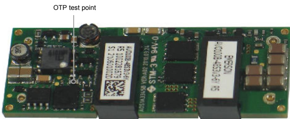
Figure 10 OTP test point
