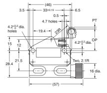
9.5 dia. × 4.0 stainless sintered alloy roller
