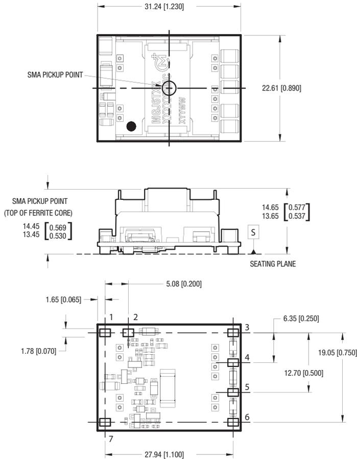
All dimensions in mm (inches), Controlling dimensions is mm.
