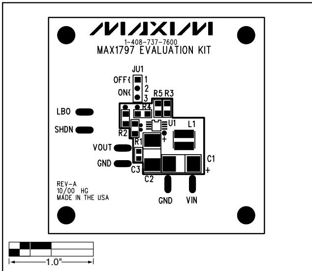
Figure 2. MAX1797 EV Kit Component Placement Guide—Top Silkscreen
