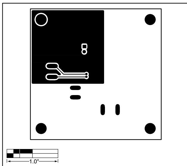
Figure 4. MAX1797 EV Kit PC Board Layout—Solder Side
