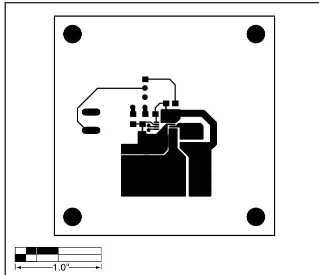
Figure 3. MAX1797 EV Kit PC Board Layout—Component Side
