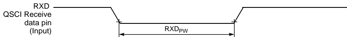
Figure 10-12 RXD Pulse Width
