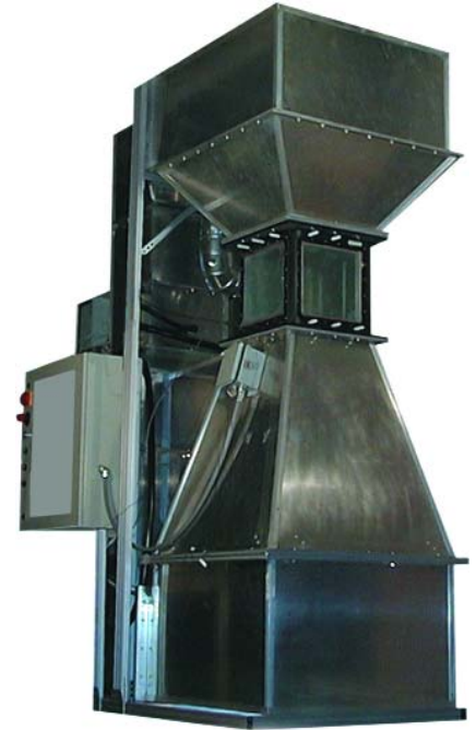
Automated temperature and velocity control
