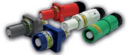
PowerLock connectors are easy to terminate to copper cable using either industry standard crimp tools or set-screw contacts. The silver plated contacts are available in 2 continuous current ranges, those with brass contacts are suitable for use up to 400 amps and those with copper contacts up to 660 amps.
