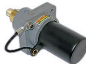
All caps are fitted with a cord lanyard for securing to it's parent connector. Cable connectors have a loop in the cord to fit around the cable gland, it is necessary to specify the cable gland size in the part number when ordering to ensure the correct size loop is supplied. Caps for panel connectors have an M6 ring terminal on the end of the lanyard.
