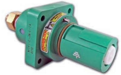
The standard connector is mounted to a panel through 4 fixing holes on the flange, panel cut-out details are shown on the right. As an alternative, the flange holes can be pre-fitted with M6 threaded inserts for either front or rear fixing, add suffix M6F for front fitting or M6R for rear fitting (rear mounting may obscure the product label, maximum panel thickness 4mm).
