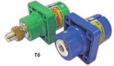
The standard connector is mounted to a panel through 4 fixing holes on the flange, panel cut-out details are shown on the right. As an alternative, the flange holes can be pre-fitted with M6 threaded inserts for either front or rear fixing, add suffix M6F for front fitting or M6R for rear fitting (rear mounting may obscure the product label, maximum panel thickness 4mm).
