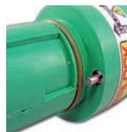
The drain connector is fitted with a secondary locking pin. When a pair of connectors are mated, the secondary locking pin engages with a slot in the source connector that prevents the connectors from being uncoupled without the use of a special release key, or when the source connector is fitted with a sliding collar.
