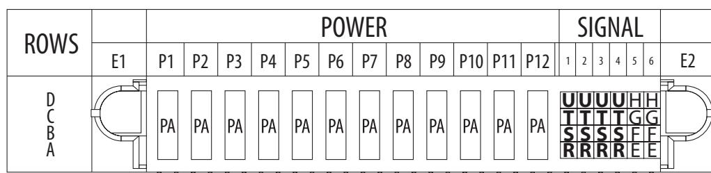
**OUTPUT CONNECTOR & SIGNAL PIN ASSIGNMENT**
