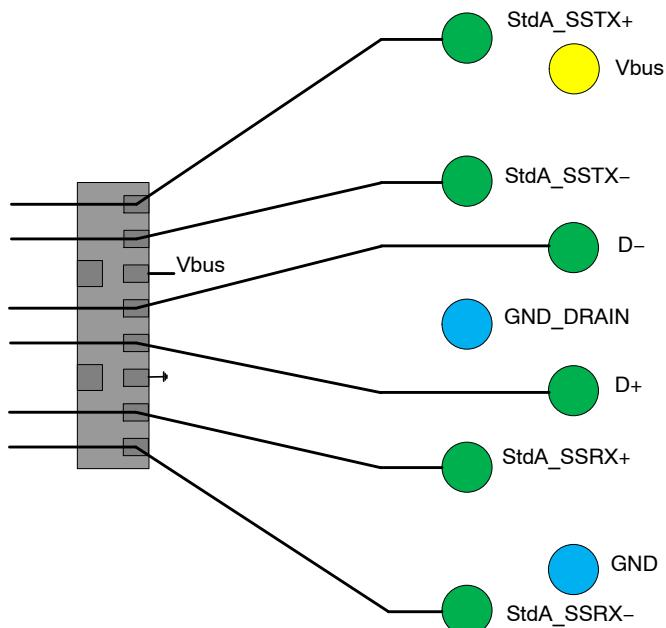
**Figure 12. USB3.0 Type A Connector Layout Diagrams**
