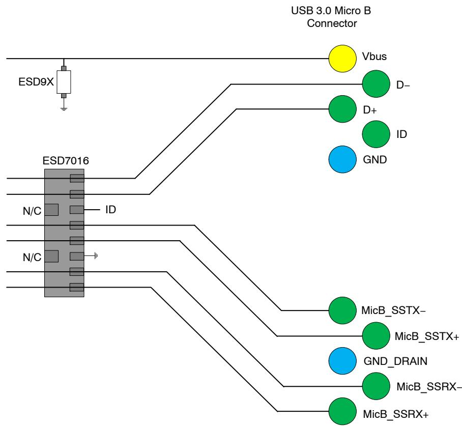
Figure 13. USB3.0 Micro B Connector Layout Diagram
