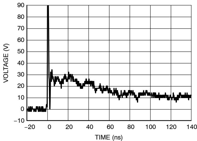
**Figure 1. IEC61000-4-2 +8 KV Contact Clamping Voltage**
