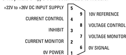
Please note: The above pin-out diagram is view looking at the connector pins.
