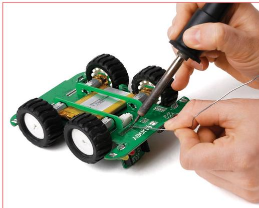
**STEP 8 -** Solder mikroBUS™ socket plates
