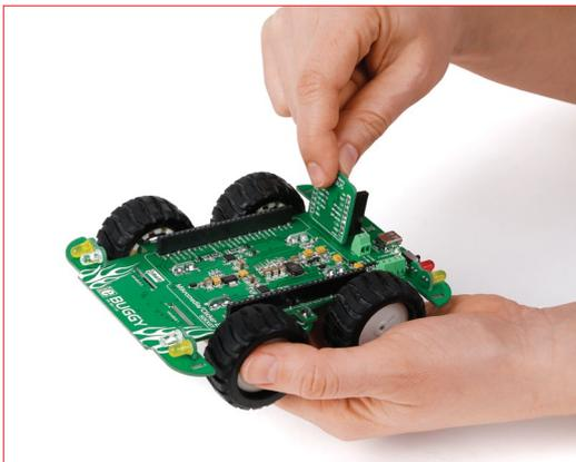
**STEP 7 -** Insert mikroBUS™ socket plates
