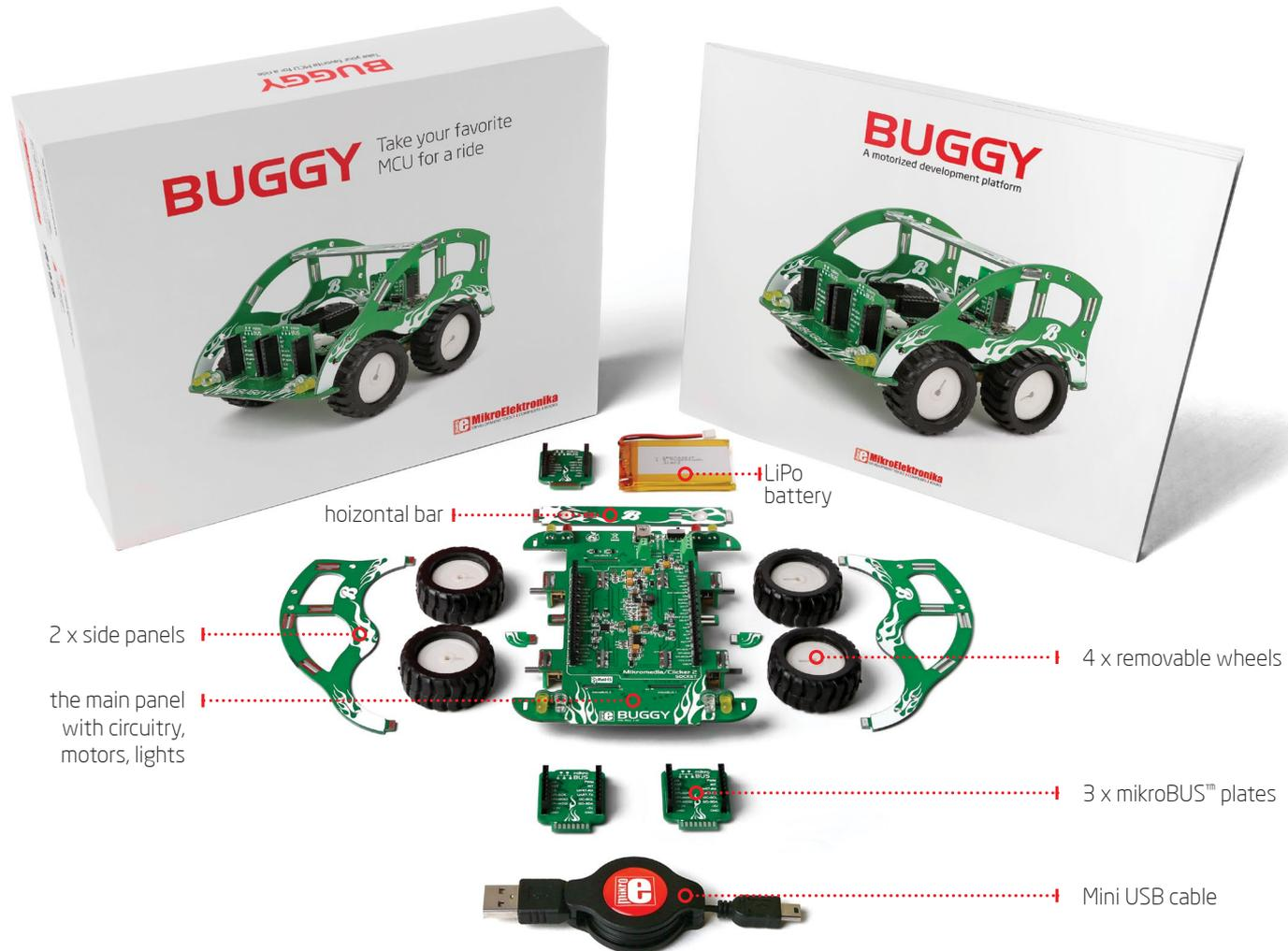
The kit contains 1) the main panel with circuitry, motors, lights, and the mikromedia connector; 2) a pair of battery holder tabs; 3) two side panels and a horizontal bar; 4) three mikroBUS™ plates; and 5) four wheels.
