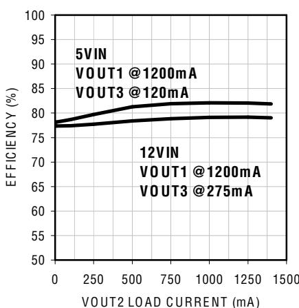
**Figure 1. Typical Efficiency of Demo Circuit 621 LT1941 with varying load current on  $V_{OUT1}$**
