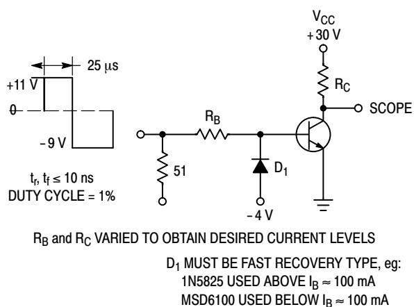
Figure 7. Switching Time Test Circuit
